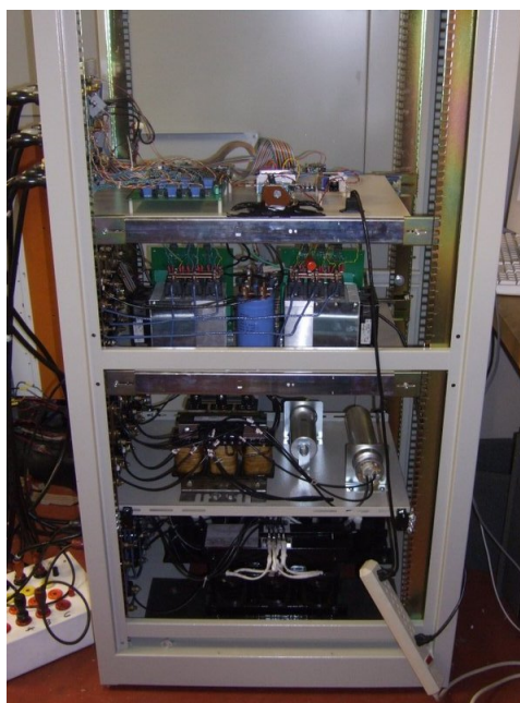
Figure 5.4: Internals of the FACTS device.
